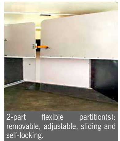
Rot-proof and noise-reducing polyethylene floor.
