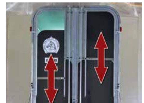
Adjustable sliding shutters integrated in the doors with 3 ventilation positions.
