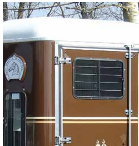
400x600 mm lateral sliding window with safety glass and protective grid.
