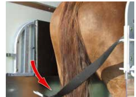
Safe release (on JMS Classic): the rear strap is releasable from the front of the trailer.
