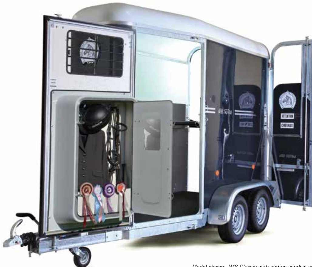
Model shown: JMS Classic with sliding window and lateral polypropylene protections.
